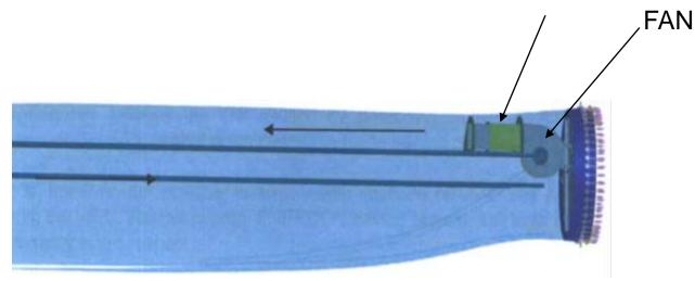
Hot air system, air circulates inside the blade
