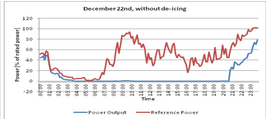
**2. De-icing warm air** 3 starts of the system, duration 6 h/cycle, 77% losses
