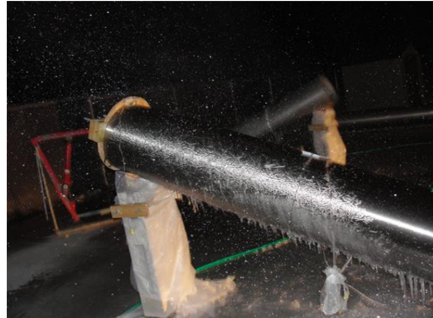
Accumulated ice in anti-icing thermal test
