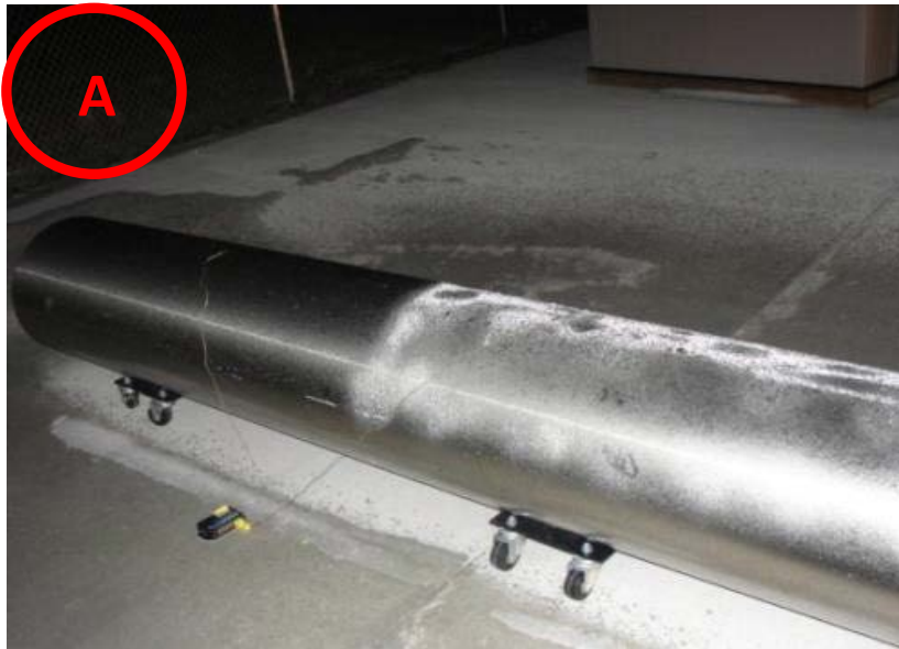
Aliphatic petroleum distillates with proprietary additives sprayed on half of the specimen
