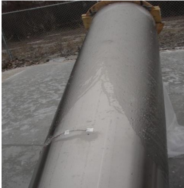
De-icing pattern in thermal test
