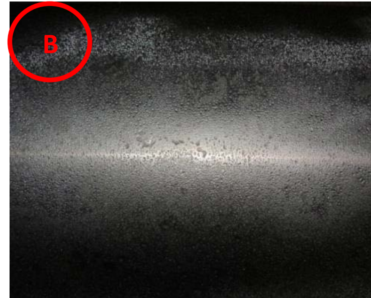
Water droplets due to icephobic coating
