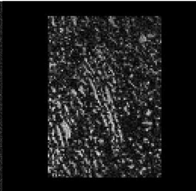
*Conventional thin section of sea-spray icing sample*
