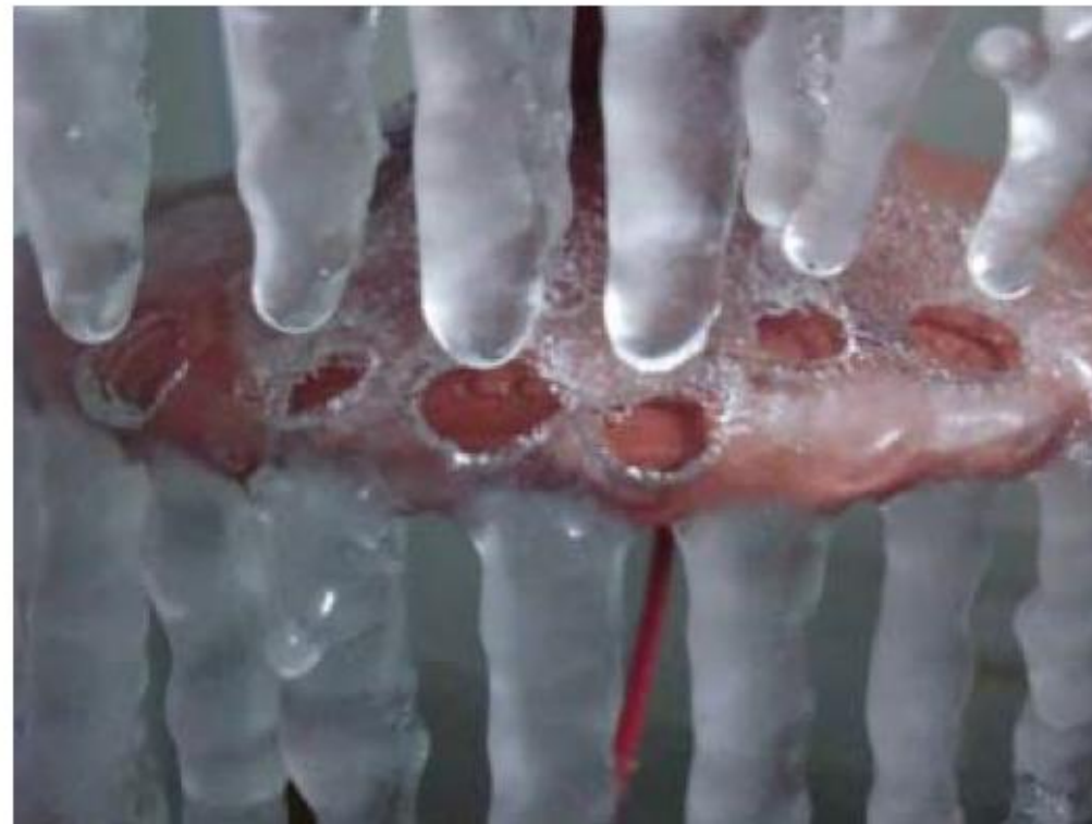
d. hollow ice layer, 1500 \mu\text{S}/\text{cm} , 20 kV
