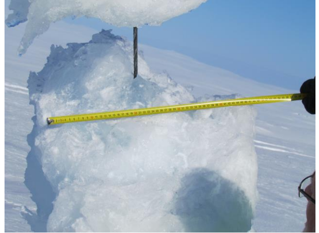
Figure 3: Ice on a guy wire in test span 00-1 after failure, the measured diameter was 47 cm.
