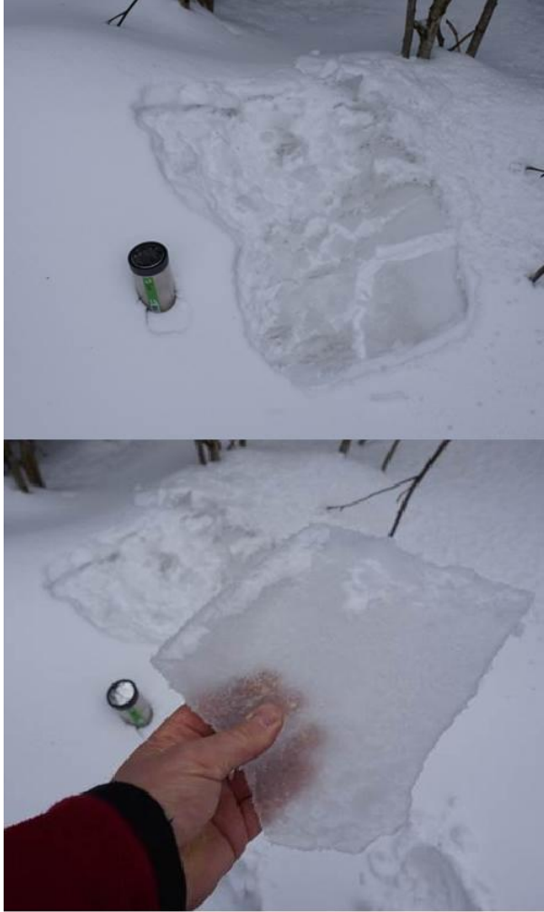
Figure 6: Icefall as 1 cm thin plate (22 cm x 38.5 cm) shed from the round top antenna of diameter 1.6 m. Picture by Amundsen, K., Norkring.
