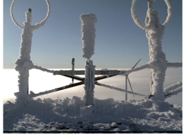
Figure 2: Example of iced instrumentation package on top of a wind turbine. Another turbine and some low-altitude icing clouds are evident in the background.
